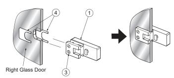
Insert the lock body (1) with the gaskets (4) into the glass door so that the gaskets will stay between the lock body and the glass door. then fasten the fixing screws 3.
