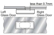
Using the adjustment of the hinges, align the glass door positions as above
