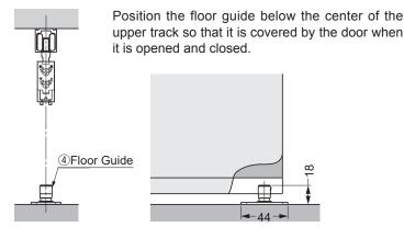
Temporarily fasten through the slotted holes with the provided screws.
