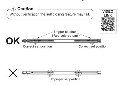
If the position is wrong, pull back the trigger catcher to the correct position using a 6 mm diameter round bar.
