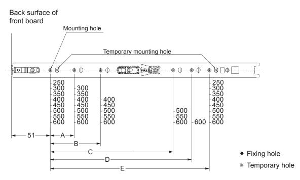
[1] Fit the inner member to the side of the drawer, either on or just below the center line for optimum stability.
