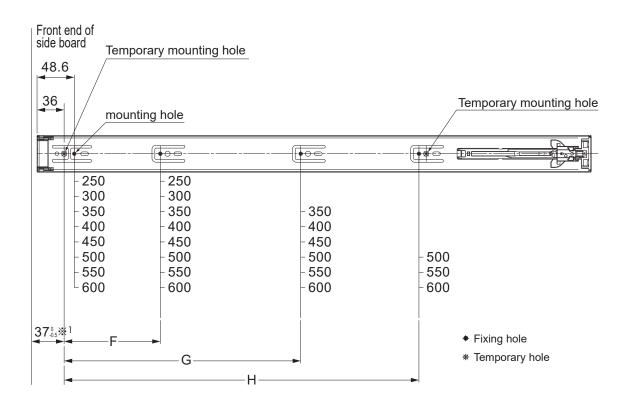
[1] Mark the positions of the slides on the inside of the cabinet and fit using the temporary mounting holes to give a little bit of adjustment.
