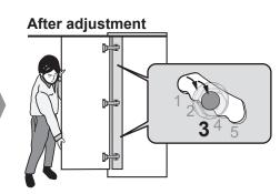
3 Tighten all the screws once the door is in the desired position.
