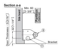
Note: Slider should always be installed towards front of the cabinet.
