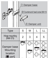
Mount the damper base and damper unit in the specified position.
