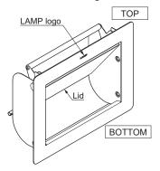
Do not leave any gap between the flap lid body and the mounting surface.
