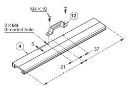
Pay attention to the direction of the end-slat and the positional relation between the end-slat and counter plate.
