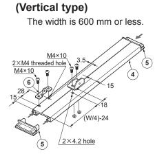
Drill threaded holes to fix the Spring plate to the end slat.
