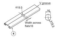
Make a hole with V-groove as the center.
