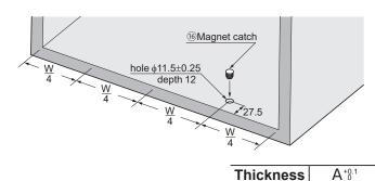
For metal cabinets, drill a hole at a position of a quarter of the opening width, as shown in the right figure.
