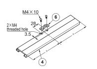
When the width is 600 mm or more, drill threaded holes in the middle of the end slat to fix the spring plate.
