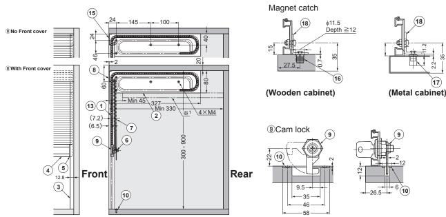
\*1 When storing unstable goods in a horizontal cabinet, it is recommended to place a middle board to avoid interference between the slats and the stored goods.
