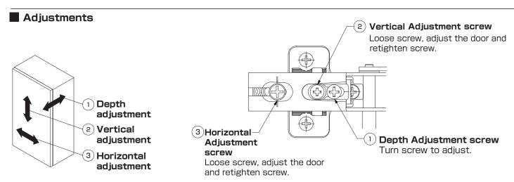
Ensure that all the screws are securely tightened. Remove all the protection tape after assembly is finished.
