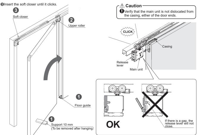
Check the position of the lever on the upper roller after inserting it into the casing.
