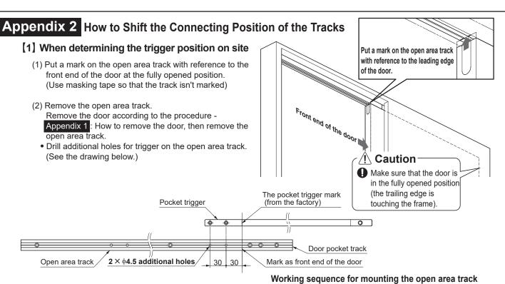
(3) Mounting open area track Follow the figure to the bottom right, since the working sequence is different from the regular process.
