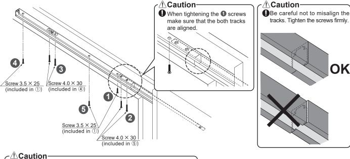
After fixing the track, move rollers and check if there is any misalignment or gap between the tracks.
