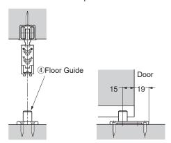
Fasten the four countersunk holes with the provided screws
