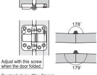
Counterclockwise (Max. 2 turns) Clockwise (Max. 1 turn)
