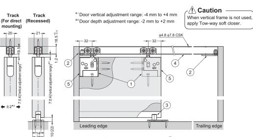
${\rm Dimension\ in\ <>:\ When\ recessed\ guide\ track \textcircled{6} under\ door\ (option)\ is\ used.}$  $\langle \ \rangle$  : When long shaft floor guide  $\ensuremath{\overline{\mathcal{O}}}$  (option) is used.
