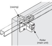
3. Door vertical adjustment (8 mm) Adjust door such that door is prallel ro upper track with 10 mm distance between door and floor.
