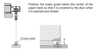
Temporarily fasten through the slotted holes with the provided screws.
