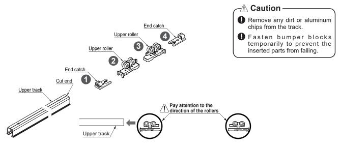
4 Mounting of Upper Track (Recommended screw: Countersunk head tapping screw 3.5×25)
