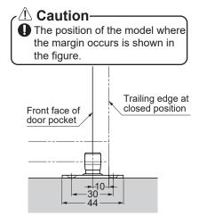
Temporarily fasten through the slotted holes with the provided screws.
