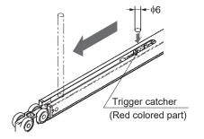
If the trigger position is wrong, pull back the trigger catcher to the correct position using a 6 mm diameter round bar.
