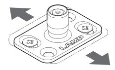
Tighten all 4 screws after the adjustment.
