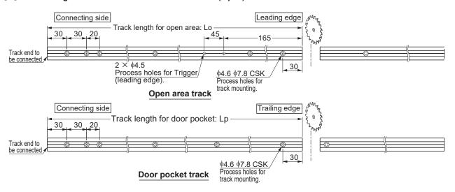
[2] When cutting from a long track (1860 mm, 2760 mm, 3960 mm)
