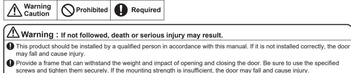
Provide a frame that can withstand the weight and impact of opening and closing the door. Be sure to use the specified
