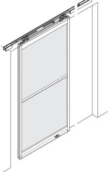
The closing speed of the soft closing type door may change depending on the ambient temperature, operating method or installation quality.
