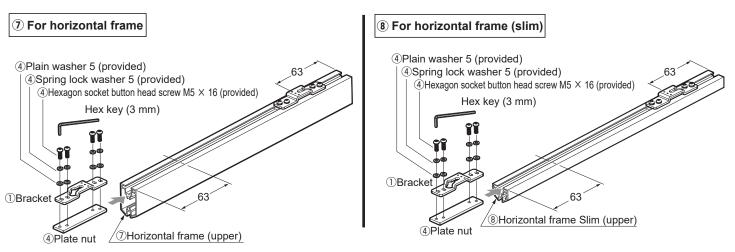
Fasten the bracket to upper horizontal frame  $(\mathcal{D}, \circledast)$ , using plate nut (4). The distance from the edge and bracket center should be 63 mm.
