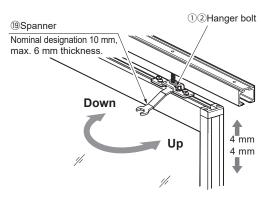
[3] After adjusting the door, pull the wrench at a right angle away from the door. Make sure the width across flats of the bolt head is as shown in the figure <sup>%9</sup>
