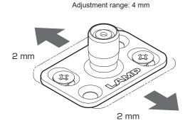
Tighten all 4 screws after the adjustment.
