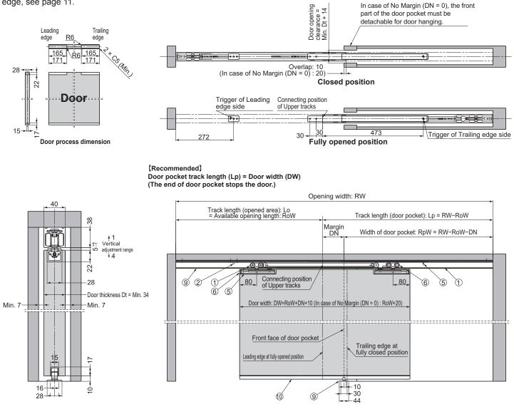
When the door pocket track is longer than the door width. (Lp > DW) (Door stoppers are needed to stop the door.)
