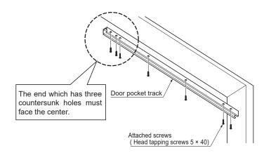
When the door pocket track is longer than the door width. (Lp > DW)
