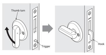
[1] While pushing the trigger, rotate the thumb turn in the direction of the arrow.
