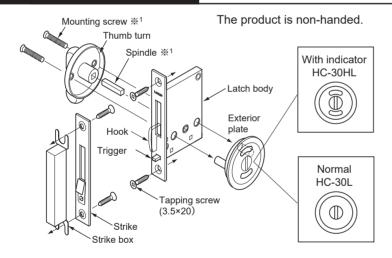
Parts to be chosen according to the door thickness (\*1)
