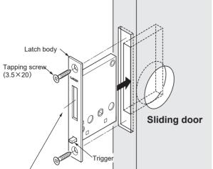
Make sure the hook is retracted in the case lock. If the hook protrudes, insert the spindle into the square hole of latch body, turn the spindle to retract the hook while pushing the trigger.
