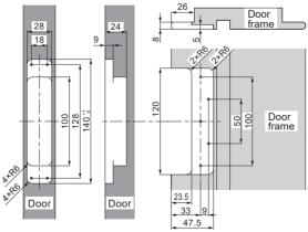
Drill pilot holes at the installation screw locations. Diameter and depth of the pilot hole depends on the strength of the wood.
