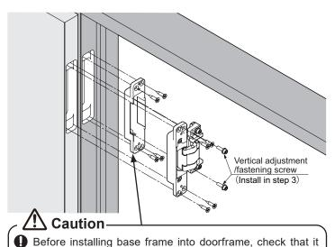
is oriented correctly. If the orientation is incorrect, the door
