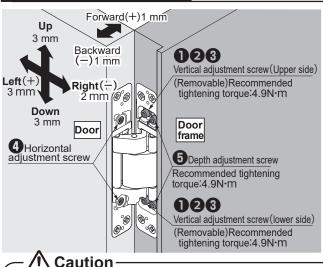
Please put a supporting spacer under the door when adjusting it.
