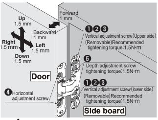
1 — 6 is the order of adjustment. Please put a supporting spacer under the door when adjusting it. There are two adjustment screws on one hinge.
