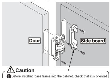
correctly. If the orientation is incorrect, the door cannot be installed.
