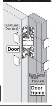
When adjusting the horizontal position, turn the two screws a little, by the same amount. The hinge may be broken if you keep turning one screw only. If you turn the adjustment screw to the right beyond the adjustment range, the parts will protrude, and the cover won't fit, and if you turn it further, the door will come off.
