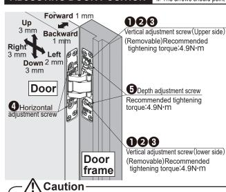
1 — 6 is the order of adjustment. Please put a supporting spacer under the door when adjusting it. There are two adjustment screws on one
