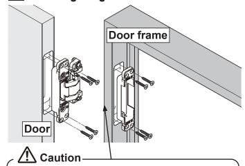
Before installing base frame into doorframe, check that it is oriented correctly. If the orientation is incorrect, the door
