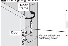
[1] Insert each hinge body (door side) deep into the base frame.
