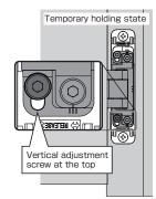
2 Raise the door to the vertical adjustment center using supports and tighten the vertical adjustment screw.
