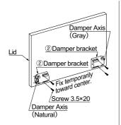
Damper Bracket [L]: Damper Axis color Natural Damper Bracket [R]: Damper Axis color Gray
