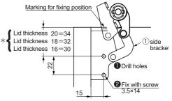
\*The above shows the rid and side board in an aligned position when the rid is closed.
