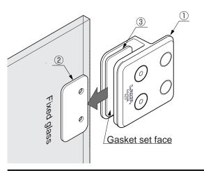
**3** .Tighten attached screws to tighten the stopper ① . Recommended torque: 1.5 N/m
