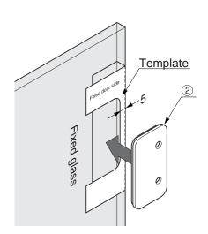
**1**.Using a template, confirm installation position. Then set rubber side of retaining plate ② to the fixed glass. Use required number of gaskets ③ in the stopper ① (refer below table).
