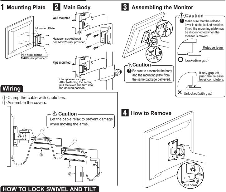
You can lock the angle of monitor when it is mounted on a slight vibrating place.
