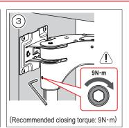
Please fasten the screws with the recommended closing torque before attaching the door.
