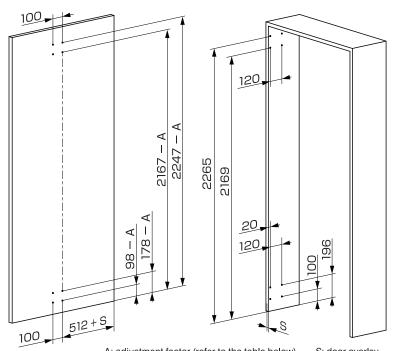
A: adjustment factor (refer to the table below) S: door overlay \*The drawing below takes into consideration a 10mm clearance between the floor and the door.
