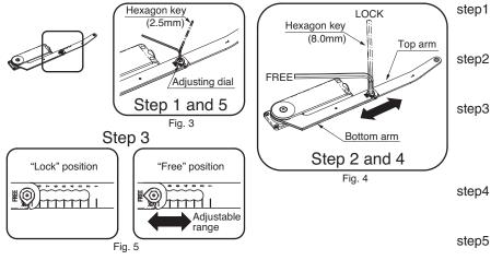
Fig. 3,4,5 Arm adjustment procedure
