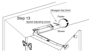
Fig. 12. Adjustment of door opening and closing speed (for right-hand side)
