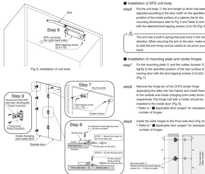
Fig. 7. Installation of mounting plate and hinges (for right-hand side)
