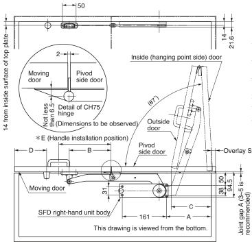
Fig. 2-1. Mounting dimensions for overlay specification (for right-hand side)
