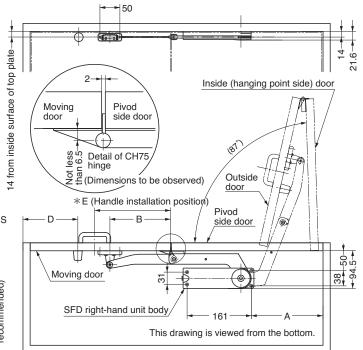
Fig. 2-2. Mounting dimensions for inset specification (for right-hand side)
