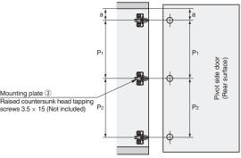
Fig.8. Fixing the mounting plates for Pivot side door
