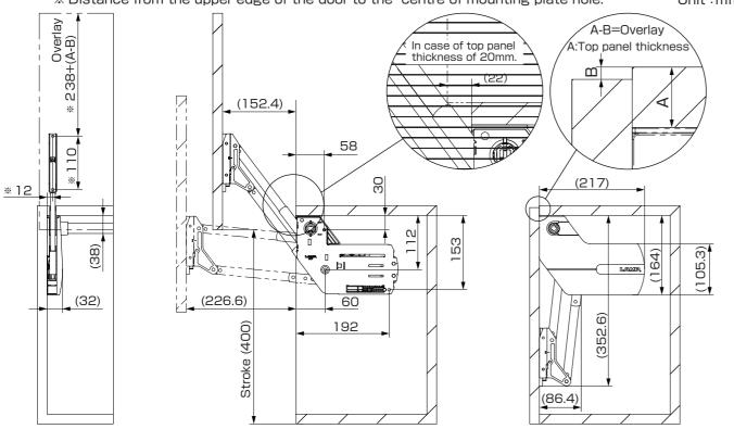
· In case of inline closely placed top & bottom doors, make sure to leave a gap of more than 3mm (if door thickness is 20mm).
