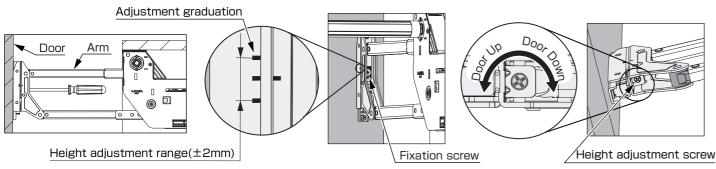
/!\ Ensure that the fixation is securely fastened.
