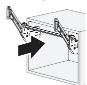
Align the grooves of the guide plate, body and push till the body is flush with the cabinet front edge.
