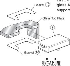
First, apply gaskets (11) to both top and bottom sides of glass top plate, and then insert top plate glass hinge support body (9).
