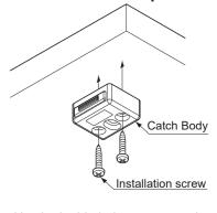
Use both side holes to secure the body catch. Size 4 screws (not included) are necessary
