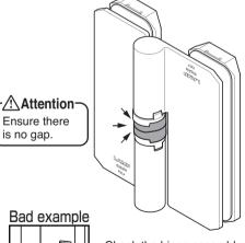
Check the hinge assembly before hanging the door. If there is a gap in the bush assembly, please turn the bush 180° and ensure that there is no more gap.
