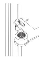
Tool: Hex key 4 mm Make sure that the clamping parts on the shelf support are fastened to both vertical frame and point fixing bracket firmly.
