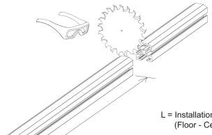
L = Installation height - 100 mm (Floor - Ceiling mounting)
