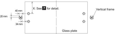
Measurement between two vertical frames (center to center): Max. 1200 mm
